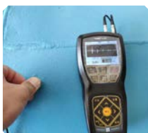
Measure through coating
